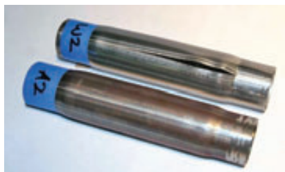
Fig. 8. Typical MSS hydroformed free-expansion burst-test specimens (upper: as welded; lower: cooling-controlled)
