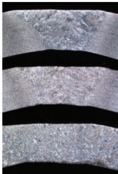
Fig. 9. MSS tubing weld photomicrographs (upper: as welded; middle: cooling-controlled; lower: Q+T)
