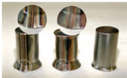
Fig. 7. Typical MSS ASTM A513 ring flare-test tube specimens (from left: as welded, cooling-controlled, cc & Q+T hardened)
